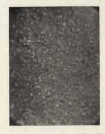
Fig. 21. (x 33 Diameters. Vertical Illumination.) Lead Etched with Nitric Acid.
